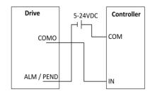
Figure 7 Sinking output
