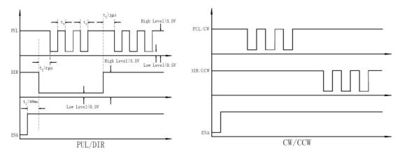
Figure 11: Sequence chart of control signals
