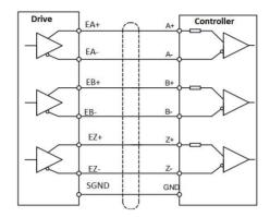
Figure 9 Encoder signals output
