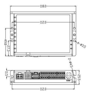
Figure 1: Mechanical specifications
