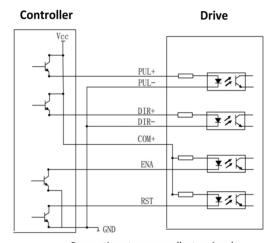
Connections to open-collector signals (Common-anode)
