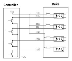
Connections to PNP signals (Common-cathode)
