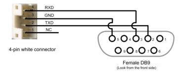
Figure 3: CABLE-PC-1 connectors
